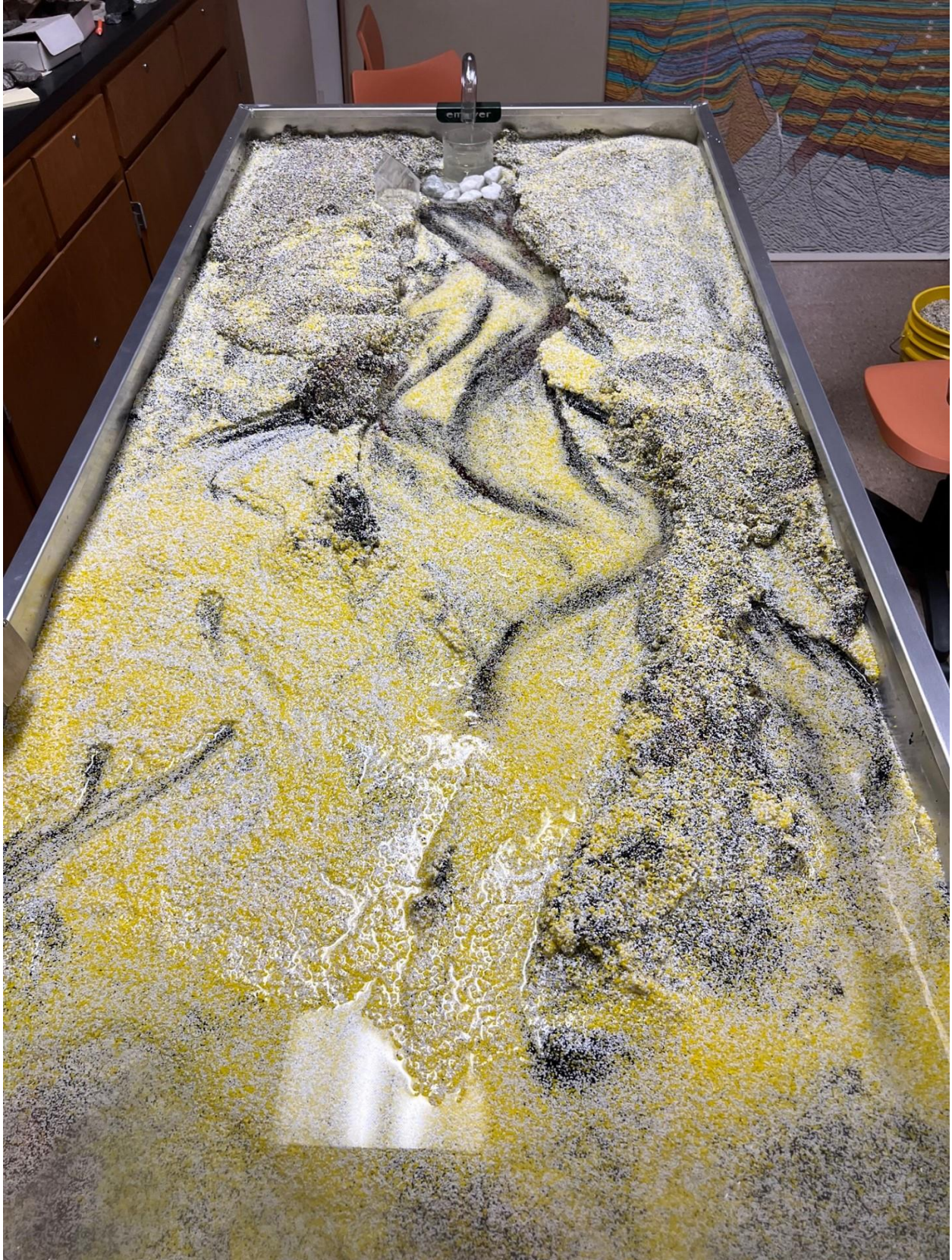
Stream table after running on initial setup showing the evolution of the river channel.
